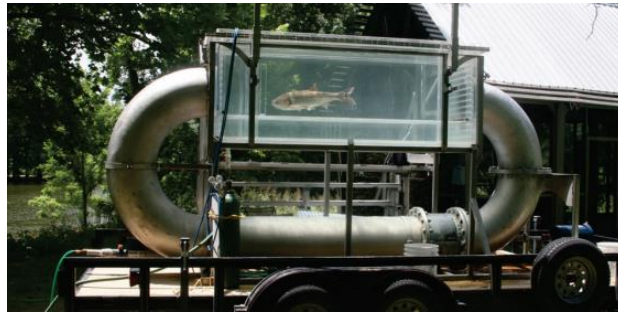
Figure 46: The mobile swim tunnel used to evaluate bighead and silver carp swimming endurance at a single velocity. Inflow was located on the left side and outflow was located on the right side with a collimator grid blocking the outflow entrance. [Taken from (Hoover et al. , 2016a)].
