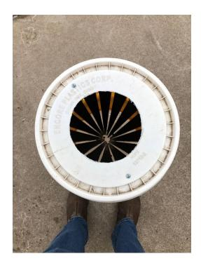
**Step #2:** You need to cut the bottom out of the top bucket. This is pretty simple to do. A lot of the area of the top bucket gets eaten up by the trap throat.
