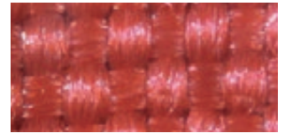
"300D POLYESTER" IceTight material under 4x magnification
